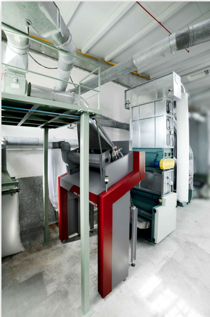
Uster Jossi Vision Shield N installed at fiber preparation for nonwovens
