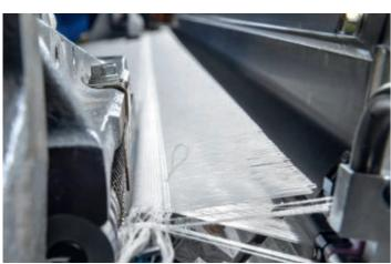
Reduce weft irregularities with weft monitoring By monitoring each inserted weft in the formation area, Q-Bar 2 allows users to react to weft
