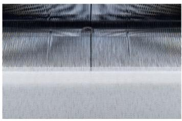
Minimize warp defects with warp monitoring With the enhanced detection position in the fabric formation zone, the warp is monitored even before it is traversed by the weft. It allows detection of incorrect warp tensioning, loose warp ends and even pattern irregularities.
