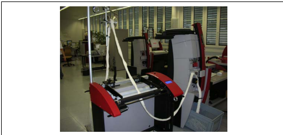
Fig. 4 Improved Unwinding Device. The feeding of sliv- er is electronically controlled
